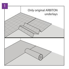
Lay the Arbiton underlay: Multiprotec LVT or Secura LVT Click Smart N perpendicularly to the direction in which panels are laid. The neighbouring ribbons of underlay must be fit tightly and joined by means of an overlap or Arbiton AluTape, without leaving any redundant space.
