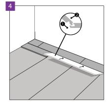
The Arbiton floor panels are provided with locks on the short and long side. First, connect the panel on the long side; for this purpose slide the long side of the panel into the groove of the previously installed row of panels. Move to the corner, leaving some clearance.
