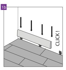
Expansion joints along the walls must be covered with a decorative strip, assembling it by means of glue or special clips. It is recommended to use the Arbiton strips dedicated to a given panel, which guarantee the excellent colour match and the coat resistant to scratching.
