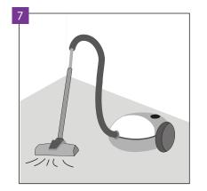
Make sure that the substrate is dry, flat, stable and free of any grease or chemical substances. The protruding irregularities must be scratched off and removed. Before the installation, the ground must be swept and vacuumed carefully so as to remove any contamination. It is necessary to repair any more serious imperfections of the substrate and large cracks.
