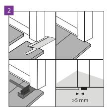
At the doors, it is recommended to undercut the profiles of door frames and leave free space over the installed panel so as not to limit its possible movement.
