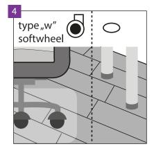
Used office chairs with W-type castors, protecting the floor additionally by means of the protective net. The furniture legs must be provided with protective pads which provide protection against scratching, e.g. made of felt.
