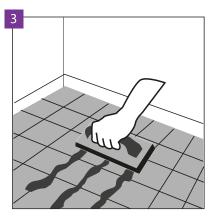
In the case of installation on the substrate covered with ceramic tiles, fill the tile joints with the gap wider than 4 mm and deeper than 1 mm with a durable compound for the filling of points, e.g. resin grout. Installation is allowed on tiles with grouts not wider than 5 mm and 1 mm deep without using levelling compound, provided the Multiprotec Hardlay or Vinclic Solid are used as underlay.
