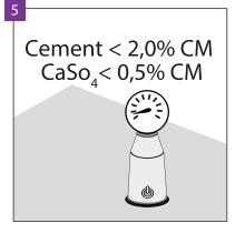
In the case of the cement grout, the moisture content in the substrate must be lower than 2.0%, and in the case of the anhydrite grout, it must be lower than 0.5%. In the case of installation with the underfloor heating, the abovementioned values must be 1.5% and 0.3% respectively.
